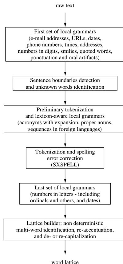
Figure 1: Overall architecture of the system.
